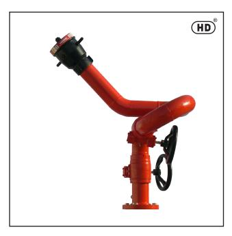
The monitor has large flow capability and can be manually operated by a single fire fighter. The design ensures to prevent jet reaction forces from effecting the horizontal and the vertical position of the monitor. The counter balance is not required to offset the weight of the nozzle. The monitor has the ability for 360 deg. continuous horizontal rotation and angle of elevation from 90 deg. above horizontal to 45 deg. below horizontal.
