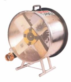
It is a high expansion foam generator. The unit consists of stainless steel casing; a pelton wheel turbine drives the fan and four jet nozzles discharge water foam solution in front of high velocity air. Foam making net is used for making foam. An inline inductor is used for inducting foam.
