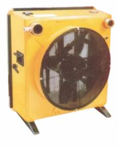
It is a high expansion foam generator. It consists of a fan driven directly by the shaft of the water turbine, which blows air to the nylon net. The net is wetted by foam water solution from the spray nozzle. The foam concentrate is drawn into the water stream by means of a built-in induction system.
