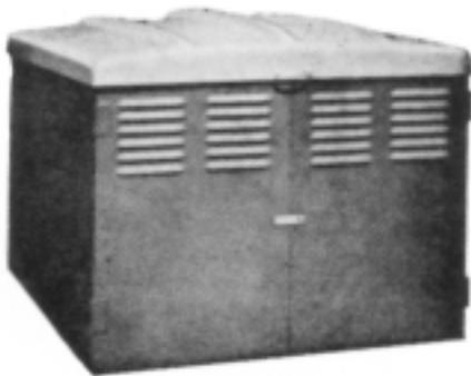
**FIGURE A-2-6.2.4(c) This type of hose house can be installed on legs as shown or installed on a wall near, but not directly over, a private hydrant.**
