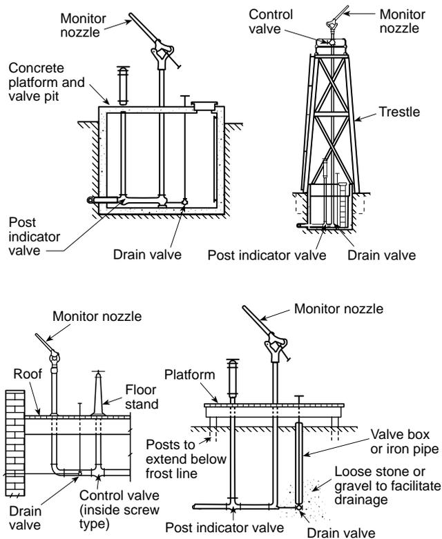
**FIGURE A-5-15(b) Typical hydrant-mounted monitor nozzle.**
