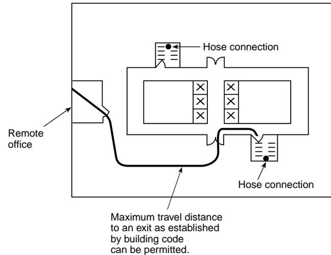
FIGURE A-5-3.2(b) Location of hose connections at horizontal exits.
