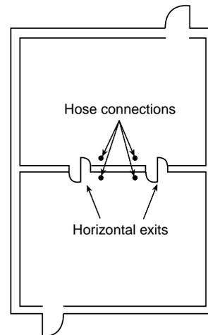
**FIGURE A-5-3.2(c) Location of hose connections in exit passageways.**
